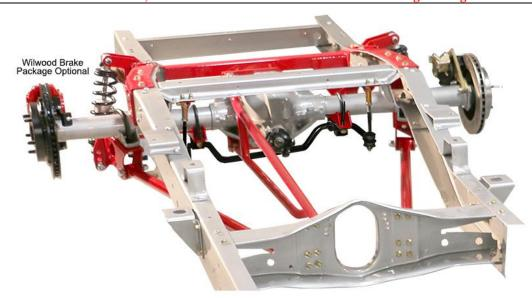
The bed must be removed in order to install these components. \*Before beginning work vehicle must be securely positioned on jack stands preferably at desired ride rake/height.
