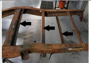
There are 3 crossmembers at the rear portion of the frame that are relevant to this installation.
