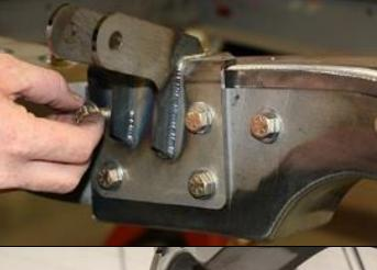
Install the 4 side bolts through the shock bracket and tighten them down to 70 lbs ft.
