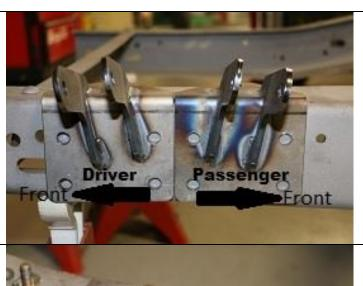
The upper shock brackets have a Driver and a Passenger side. Once placed onto the frame in the correct position the shock mount brackets will sit vertical.
