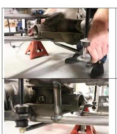
With the top bushing and cupped washer in place you can now lift the anti-sway bar up into place making sure the studs line up with the holes on the bar.
