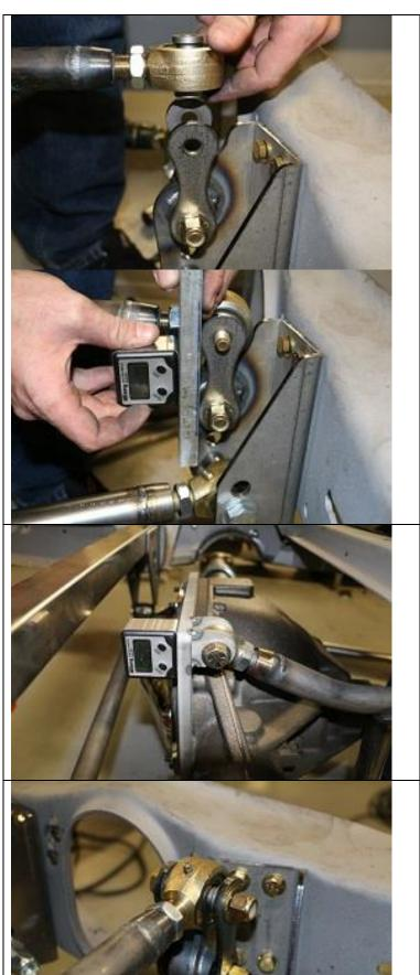
The Dog Bone needs to sit vertical with the Torque Arm attached and the rear axle at ride height. Make adjustments as needed.
