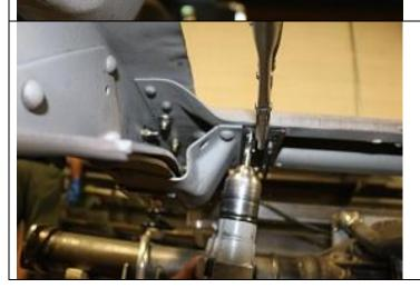
Place a vise grip or c-clamp on the bracket to hold it in place. Drill the remaining 3 holes and install hardware loosely.
