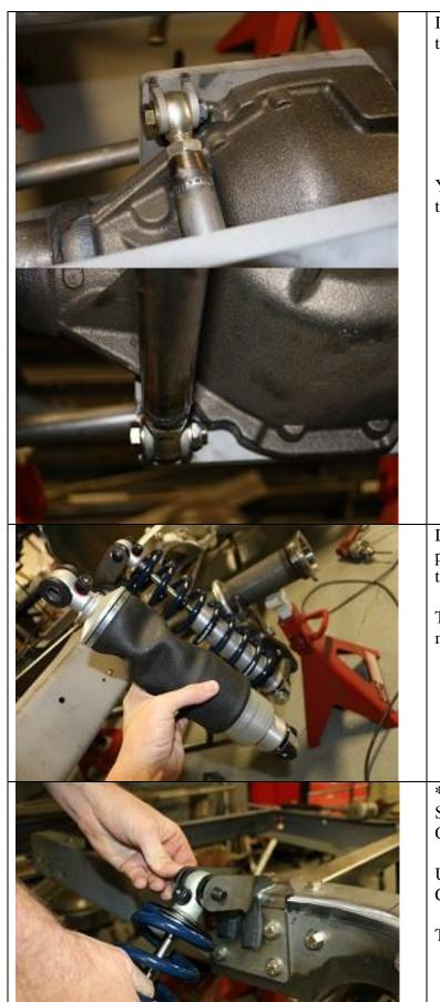
Install the hardware on the Torque Arm plate and torque to 70 lbs ft.
