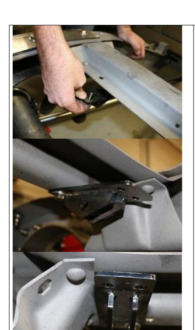
On the driver side of the factory shock crossmember there is a single hole on the back side we will be using. The bolt installs from the bottom going up.
