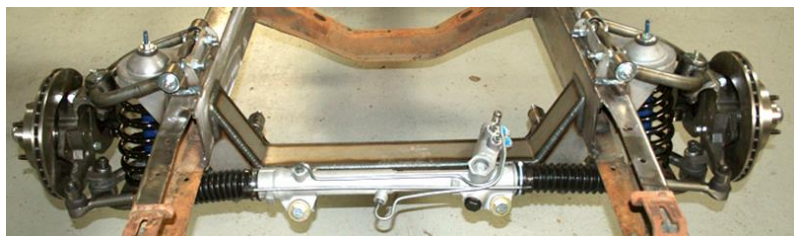
New Coil-Spring Front End on Original Stock Chassis
