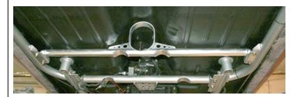
If the optional sub-frame connectors and driveshaft loop were purchased they are installed next. The driveshaft loop cross-member is installed under the brackets on the connectors using the  $3/8 \times 1$  inch bolts, nuts and washers. Center the loop in the driveshaft tunnel before tightening.
