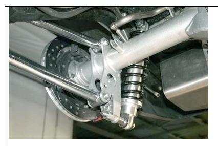
Next the rear axle assembly has to be installed. It's a lot easier to install the bare housing and install the  $3^{rd}$  member, axles and brakes later but that's your choice. First, install the coil-over's on the front of the top cross-member using the  $5/8 \times 18 \times 4^{1/2}$  bolt, washer on each side of the shock bushing then the 5/8" spacer against the cross-member and the full nylock nut on the back.
