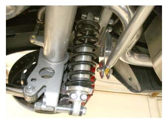
The photo on the left shows the panard bar attached to the axle housing bracket using  $\frac{1}{2}$  x 20 x 2 inch bolt, washers and Nylock nut. The process is repeated on the right side on the panard bar bracket that is bolted to the coil-over cross-member. The three hole adjustment gives the choice of raising or lowering the rear roll center. Finish the project by installing the shock hole block off plates using the four 5/16 x 18 x 3/4 button head bolts.
