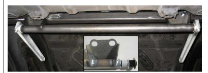
Mount the 4-link bars into the frame bracket using the button headed  $5/8 \times 18 \times 2^{3/4}$  bolts with the stainless adjustors forward in the frame bracket. Tighten the ½ nylock nuts and position bars to accept rear axle housing.
