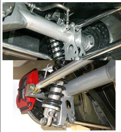
The sway bar is connected to the axle housing brackets with a  $3/8 \times 1^{1/4}$  inch button headed bolts. The link is tapped 3/8 inch left and right for ease of adjustment while still bolted up. The sway-bar end uses a lock washer and the bracket on the axle housing a nylock nut.
