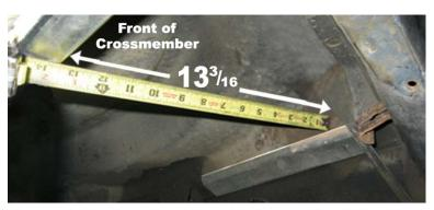
Next using the 5/16 inch bracket holes as a guide, drill one 5/16 hole through the floor pan and install one of the  $5/16 \times 1^{1/4} \times 24$  button head bolts and install nut on inside and tighten. This will keep the bracket from moving around while drilling and all holes will line up when finished. Finish drilling remainder of the holes using a long shank 5/16 inch drill bit.
