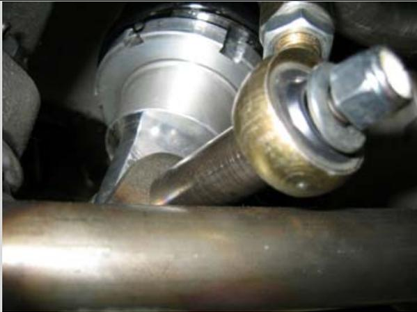
**Next, install the shock into the lower a-arm tabs making sure that the adjustment dial towards the rear of the vehicle and install the 3  $\frac{3}{4}$  inch shoulder bolt from the rear through the rear bracket, then the shock bearing, front bracket, then the spacer and last the rod end link for the sway bar. Install the washer and nut and tighten. The top rod end will be attached to the sway bar later.**
