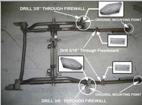
Start the installation of the new sub-frame by raising it up into the original mounting position. A floor-jack will help here. Line up the holes in the firewall and the far rear mounting point and fasten it using the new supplied bolts, lock washer and flat washer (Qty. 4 5/8-11 x 2" Gr. 8 Hex Head) Using a 15/16" shallow socket. Do not tighten up the bolts at this time until all mounting bolts have been started then tighten and secure to the body.
