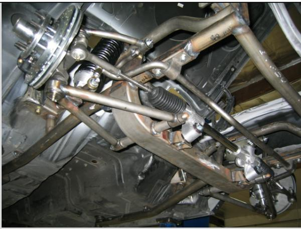
**Make sure all fasteners are tightened to the recommended torque specifications and you have completed the assembly of the TCI front suspension.**
