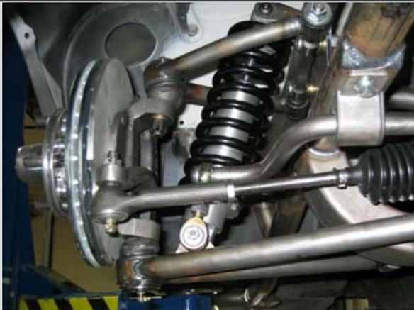
**The spindle assembly is installed next. Set the spindle assembly on the lower ball joint with the steering arm facing forward and the brake caliper towards the rear. Install the lower ball joint nut, tighten and install cotter pin. Pull the upper a-arm ball joint down into the top of the spindle and install nut, tighten and install cotter pin.**
