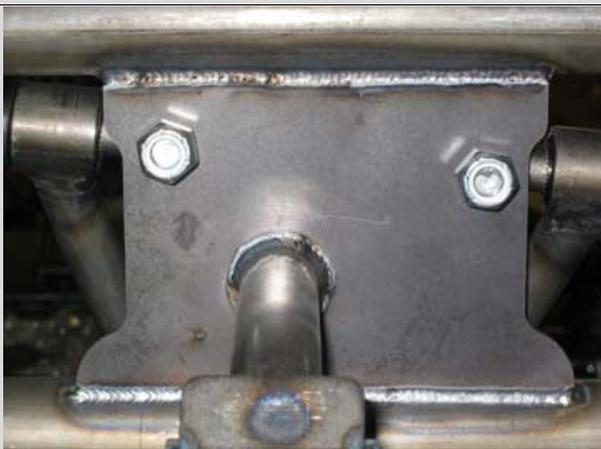
Complete installation by tightening the supplied 9/16-18 full height Nyloc nut.
