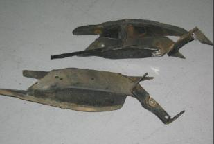
If a TCI anti-sway bar package is being installed go ahead and cut off the stock sway bar brackets and the strut rod support channels.
