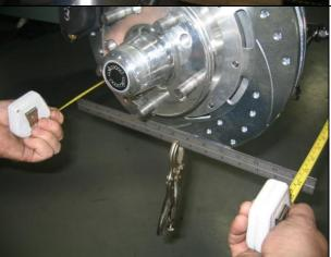
Clamp a straight edge to each rotor as shown then using a tape measure front and rear; set the toe-in approximately 1/8" for a starting point.
