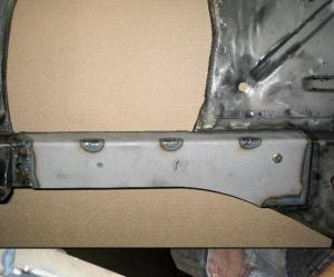
Weld the inside boxing plate on the top, ends, sides and rosettes.
