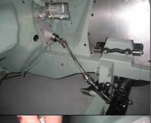
The rack will have to be unbolted and slid forward to install the shaft.
