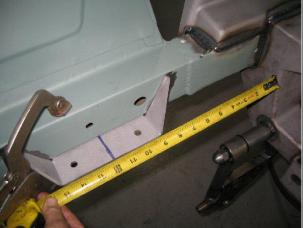
The sway bar bracket is mounted 12 inch's from the front edge of the cross member to the center of the bracket.
