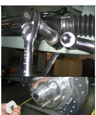
Install the rack using the two 5/8" bolts, washers and nylock nuts with antiseize on the threads and tighten.
