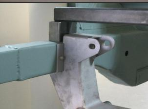
Next slide the cross member (steering rack brackets forward) between the rails behind (firewall side) the locating plates.
