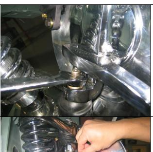
The spindle and brake assembly comes completely assembled with the bearing's packed and seals installed and is installed next. With the steering arm forward and caliper rearward set the spindle onto the lower ball joint and install AN washer and nut, tighten and cotter pin.
