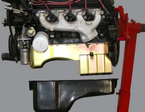
All engine installations with this front end will require a fox body rear sump oil pan small and big block applications. 289-302 Small Block Ford Motor
