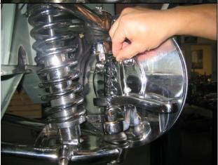
Install the top a-arm ball joint into the spindle. Install AN washer and nut. Tighten and cotter pin.
