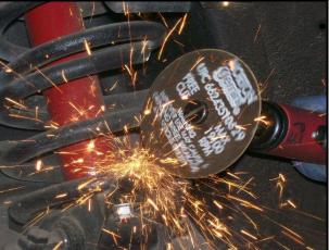
Remove all the old suspension components including the steering column. I used a die grinder with a cut off wheel to cut the coils in a couple of places for much easier removal.
