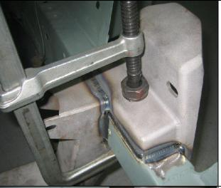
Use a C-clamp from the inside and pull the bracket down snug to the top of the frame rail.
