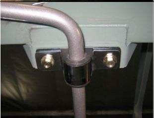
Install the sway bar (center drop of bar down) next using the four 3/8" bolts, washers and nylock nuts. The spacer plate goes against the frame bracket first then the saddle bracket next.
