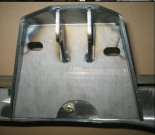
The a-arm/shock tower bracket is mounted with the highest a-arm bolt slot forward and the lowest slot rearward.
