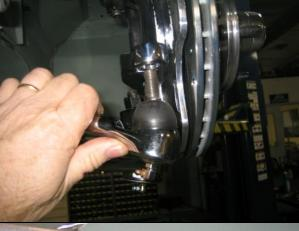
Install the tie rod end jam nut and then the tie rod end turning it an equal amount of turns per side until they line up with the steering arm tapered hole. Check the toe-in again, adjust if needed.
