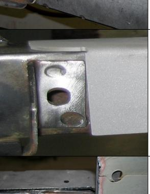
If the stock sway bar bracket was not removed, you will have to notch the inside flange one inch back for the locating holes to line up.
