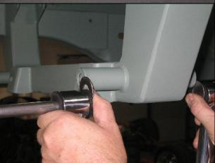
The lower a-arms are installed with the sway bar bung facing forward. The 5/8 inch shaft is installed with the acorn nut facing forward with a thin stainless washer on both sides of the urethane bushings on the a-arm.
