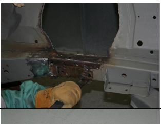
Remove all excess material, welds and paint from the main rails to all for the installation of the boxing plates.
