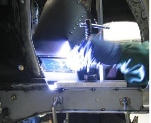
It's time to tack weld inner and outer boxing plates to each other and to the frame. When it comes to welding, I prefer to heli-arc because it's cleaner and less grinding afterwards but a wire feed will work fine, just a little more clean-up grinding afterwards.
