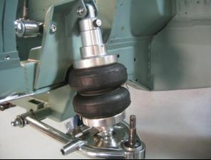
When using Shock Waves with a spherical bearing, a provided spacer will be required on each side of the spherical bearing.
