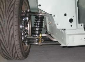
Proper ride height is with the lower a-arm level to the ground. Adjust the height with the threaded ring on the bottom of the coil-over.
