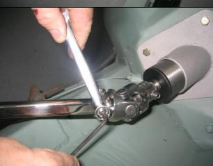
Loctite the set screws before tightening and loctite the jam nuts.
