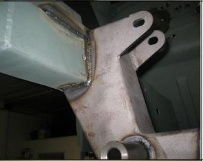
Double check for square and tack weld all sides and on the bottom.
