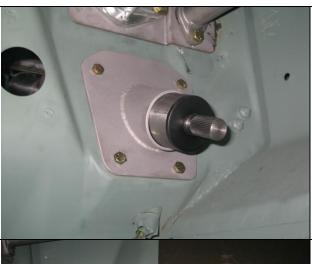
With the column installed, put the Borgenson universal joints onto the end of the column and the pinion on the rack. The power rack and the column were both  $^{3}4$ "-36 spline X  $^{3}4$ " DD.
