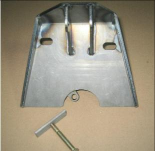
It is critical that the two edges are parallel even if you have to trim off of the bottom edge of the outside boxing plate.
