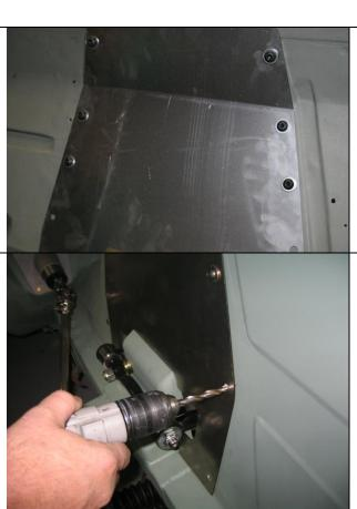
Position the correct panel over the a-arm until the bolt holes line up. The are three on each side of the panel with the existing stock inner panel holes.
