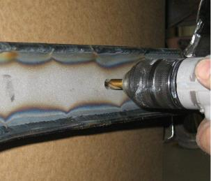
Drill the frame through from both sides in the 3/8" hole in the boxing plates to make the locating point.
