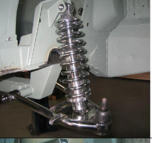
The shock assembly is installed next using the ½ inch bolts.
