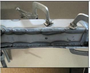
Using the outer edge of the lower boxing plate as the template, grind the two stock frame flanges till they match the profile of the boxing plate edge.
