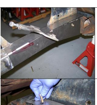
You are now ready to start installing the boxing plates to strengthen the frame in the cross member area.
