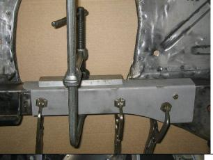
After clamping boxing plates using support plates double check to make sure plates are flat on the frame rail and as close to 90 degrees as possible to each other.
