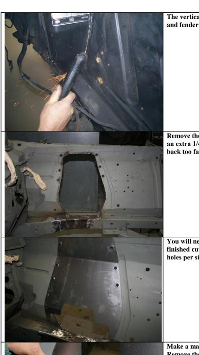
The vertical cuts on the towers are made at the bend radius between the tower and fender panel.
